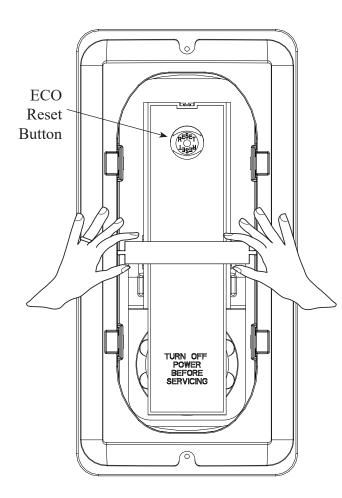
In order to replace the ECO, thermistor or heating element, remove the cavity insert crossbar by following the instructions below:
