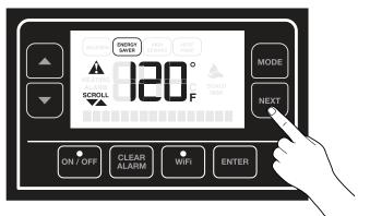
2) Press "Down" arrow button to scroll through the active alarms.
