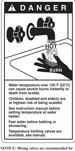
NOTICE: Mixing valves are recommended for reducing point of use water temperature by mixing hot and cold water in branch water lines. It is recommended that a mixing valve complying with the Standard for Temperature Actuated Mixing Valves for Hot Water Distribution Systems, ASSE 1017 be installed. See page 16 for more details and contact a licensed plumber or the local plumbing authority for further information.
