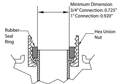
The hot water connection fitting must have an inside diameter greater than the minimum shown in the picture above.
