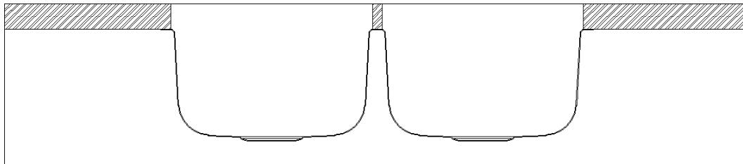
**Flush** - The countertop meets the edge of the sink. Fitting flush with the sink bowls
