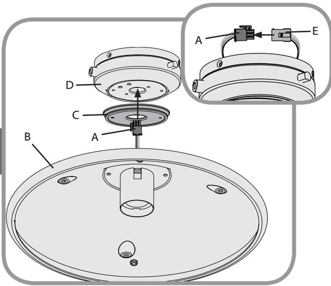
Thread the plug connector (A) from the light kit (B) through the adapter (C) and through the bottom of the lower switch housing (D). Connect the plug from the light kit (A) to the plug from the switch housing (E).
