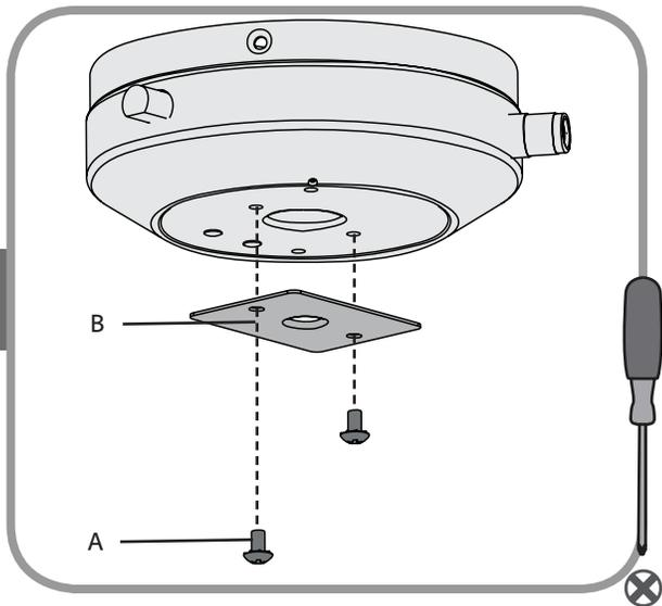
If present, remove the plate screws (A) and the plate (B). Go to step 8 on page 6.
