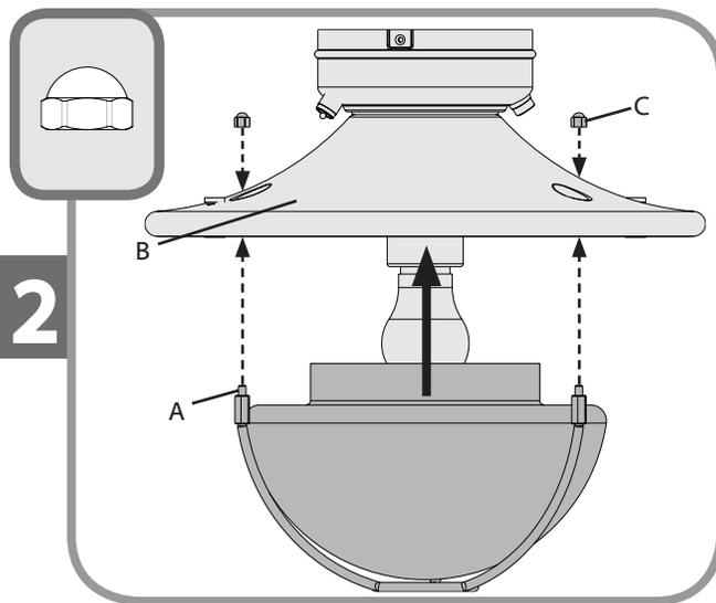
To reinstall the globe assembly, align the posts (A) on the globe assembly with the holes in the shroud (B). Make sure that the chain holes in the globe assembly also line up with the chain holes in the shroud. Lift the globe and posts until the threaded end of the posts are visible through the shroud. Install the three acorn nuts (C) onto the posts so that the light kit is secured to the shroud.
