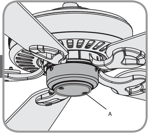
If your fan's switch housing cap has two visible screws (A), go to step 6 on page 5.
