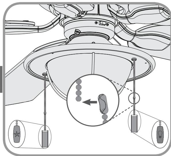
Connect the appropriate pull chain pendant to each of the short chains. The fan pull chain (B) controls the speed: from high to off. The light pull (A) chain controls the light fixture: on and off.
