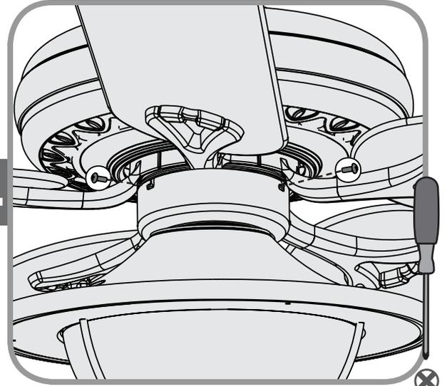
Lift the lower switch housing until its screw holes are aligned with the screw holes in the upper switch housing. Install the 3 switch housing screws you saved. Tighten all three screws.
