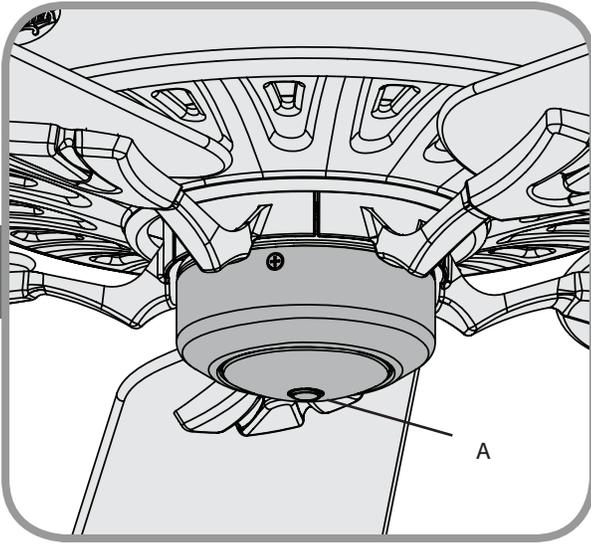
If your fan's switch housing cap has a plug button (A), go to step 3 on page 4.
