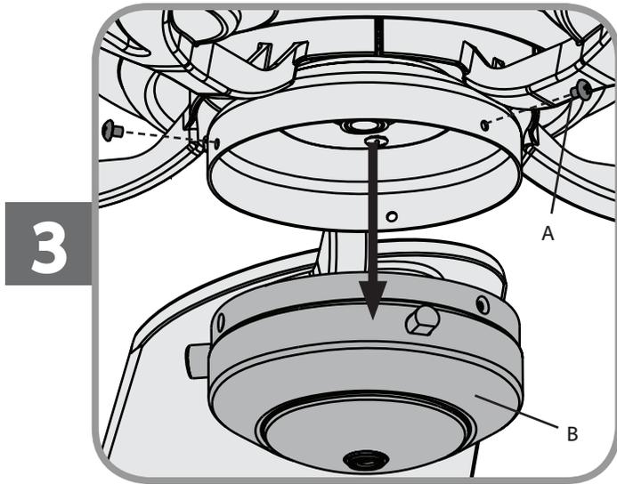
Remove the 3 switch housing screws (A). **SAVE THE SCREWS.** Lower the switch housing (B).
