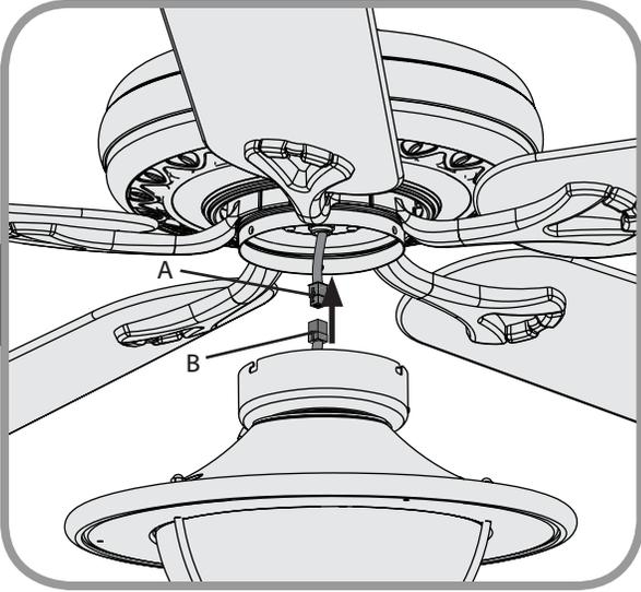
Connect the plug from the upper switch housing (A) to the plug from the lower switch housing (B).
