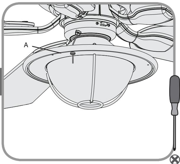
Feed the chains from the fan and the light switch down through the holes in the shroud (A).
