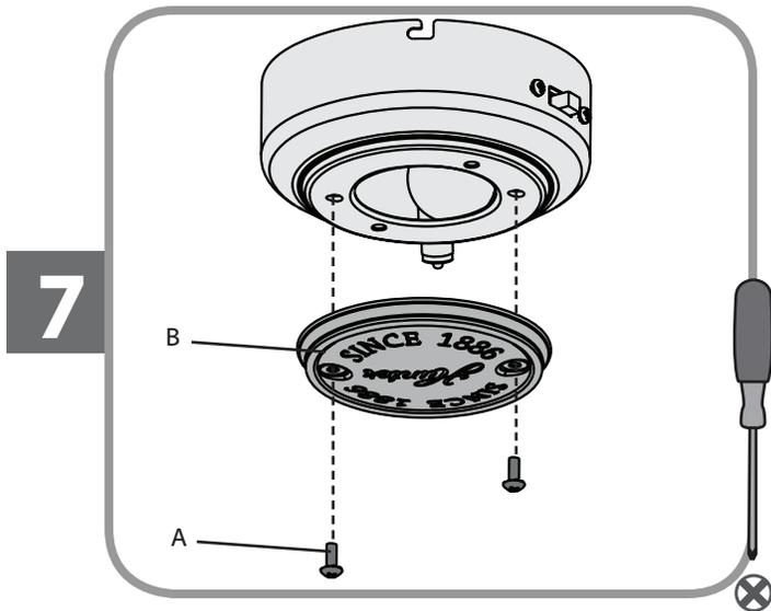
Remove the switch housing screws (A) and the switch housing cap (B).
