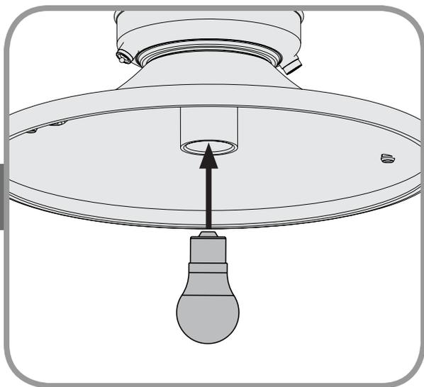
Install a bulb (A) into each of the sockets. When necessary, replace with bulbs of same wattage.
