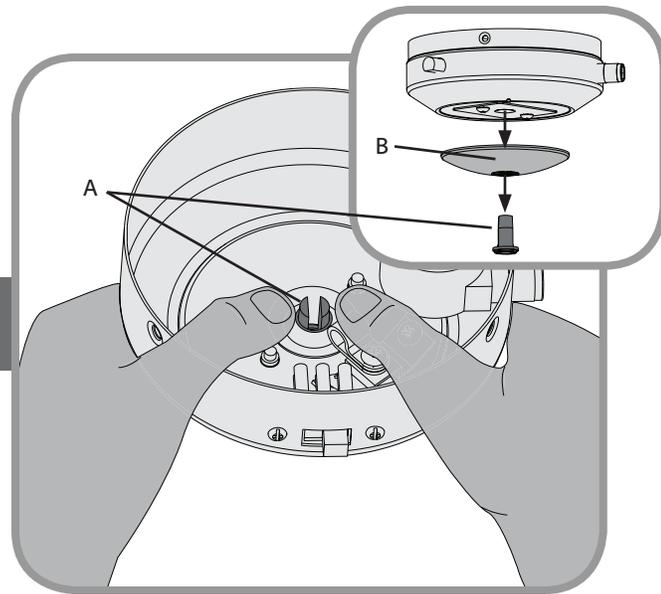
Push the plug button (A) and switch housing cap (B) out of the bottom of the switch housing.
