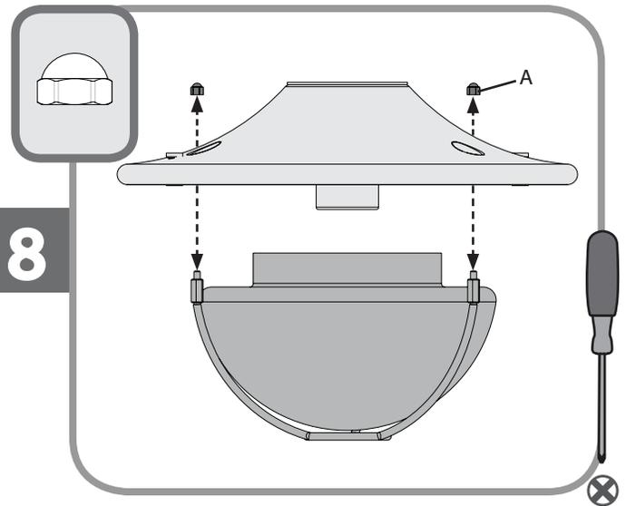
Unscrew the three acorn nuts (A) by hand and carefully detach the globe assembly from the shroud. **KEEP THE ACORN NUTS.**
