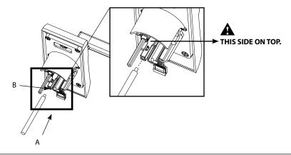
**Step 2:** Position the Outside Trim Plate Assembly through the bore hole.
