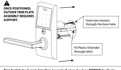
**Step 3:** With the Outside Trim Plate Assembly flush to the door, *REMOVE* the Plastic Extender.
