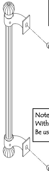
Use flat head screwdriver to install 3/8-16 threaded inserts (provided) Flush to Handle.
