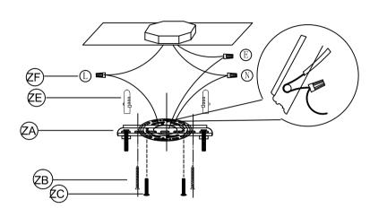
1. Drill two holes on the ceiling and put the plastic anchor screw(ZE) into the holes(If the wall is wood made, this step can be ignored); 2. Attach the Bracket (ZA) to the Junction Box with two screws(ZC).
